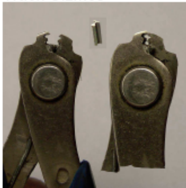
Rail shear made from pliers, notch matches rail, open, ready to shear, inset is sheared rail as cut
