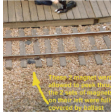
Ballasting can hide the magnets
