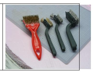
Wire brushes are used to take the foam board that has been cut to the final stage of developed scenery. Wire brushes are good for howling out indentations, creating exposed rock on the sides of cuttings, smoothing the tops of hills and creating fields, streams and rivers. Brushes are made
