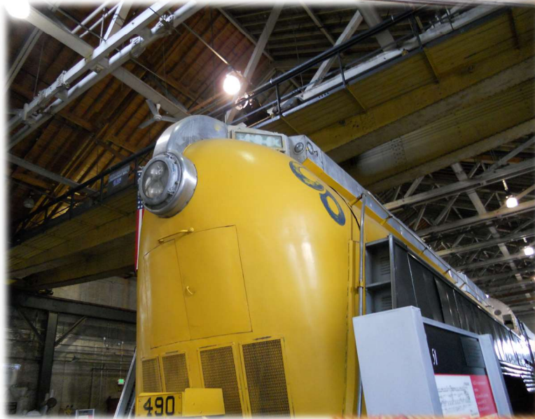
1926 Chesapeake and Ohio #490 2-6-2 "Pacific" Rebuilt in 1946 into Class L-1 Hudson 4-6-4
