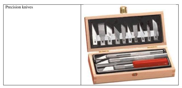
5. Precision knives are used to add texture to the sides of a cutting to add rock detail. I cut into the side of cutting using the knife, making horizontal and vertical cuts to bring out the rock detail I am trying to model. This is done after the brushes have been applied to give the overall effect.
