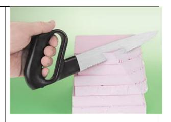
Keyhole saw which can be found at hardware stores, Home Depot, Sears, in fact, any place that sells tools. This saw is used for cutting holes in sleet rock and wood. It can be used like the foam board saw. The teeth are larger in this saw so they tear up the foam board more so be careful. Otherwise you will remove more material than you intend to remove.
